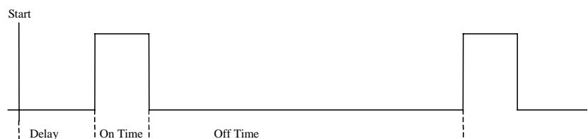
Fig. 3-5 Trigger delay, on and off times for SMIQB60 trigger.
